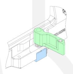
3. Rotate (loosening/tightening the clamp)
