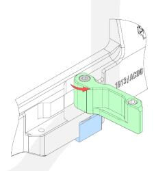
2. Elevate (decoupling with the locking bolt)
