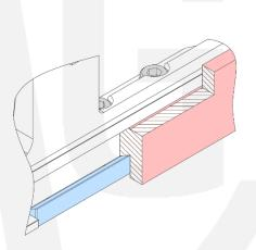
□ clamping bar □ M5 bolt □ 4 mm hex key □ side rail
