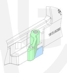
□ rotating lever □ clamping bar □ proprietary locking bolt
